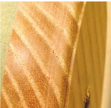
▲ Pic.16 This close-up shows you the fine detail that can be achieved with high speeds and sharp tools. Very small details are impossible to sand without ruining the shape
